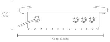
Lux Button Push In, Light On At Night, Push Out, Always ON 850nm Button Push In, 850nm wavelength IR On, Push Out, IR OFF 940nm Button Push In, 940nm wavelength IR On, Push Out, IR OFF
